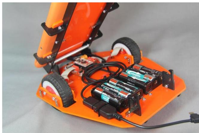
To access the batteries remove the tablet by lifting it from the rear of the robot.
